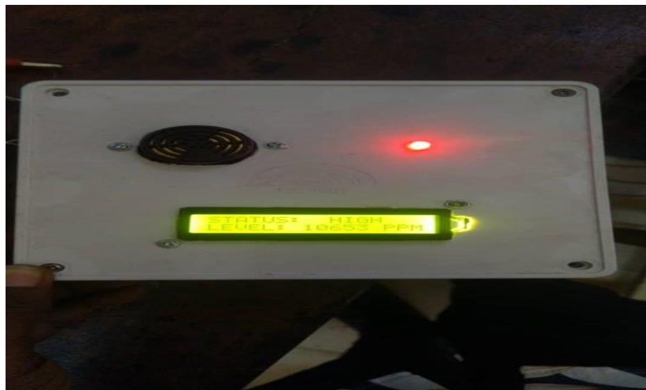
Figure 4. Constructed detector undergoing test when the carbon monoxide concentration is above the set limit.
