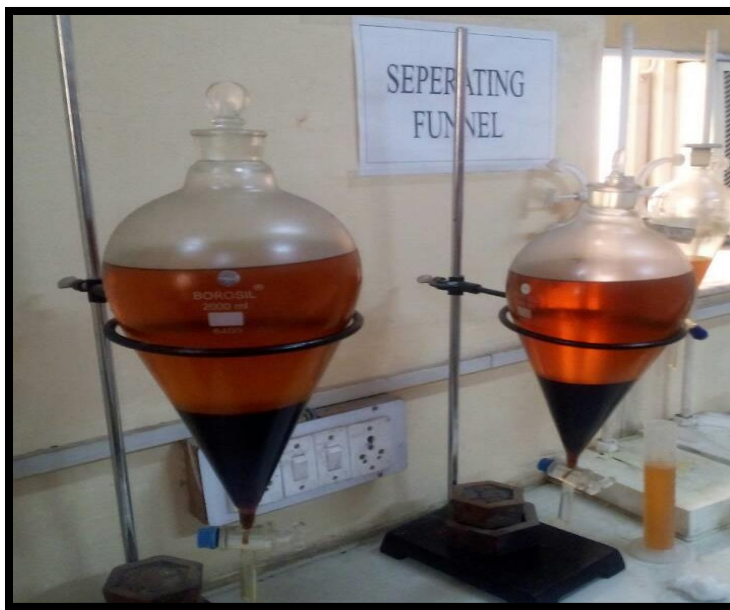
Fig 1: Separation of biodiesel in separating funnels using base catalyst
